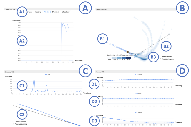
Figure 4: The Module Tabs: A Perception tab which contains a navigation bar (A1) and a line chart (A2) that displays the selected metric of the object; B Prediction tab which aggregates the predicted trajectories of the object; C Planning tab which utilizes DTW (Dynamic Time Warping) to determine moments with sharp changes in planning; D Control Tab which displays line charts for throttle (D1), brake (D2), and steering (D3).
