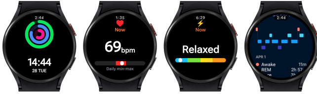
Figure 3: Visualization examples on Wear OS smartwatches implemented using SalusChart’s :wear module. From left to right: an activity ring showing daily goal progress, a heart rate display with daily min–max range, a multi-segment gauge indicating current stress level, and a sleep stage chart summarizing recent sleep.
